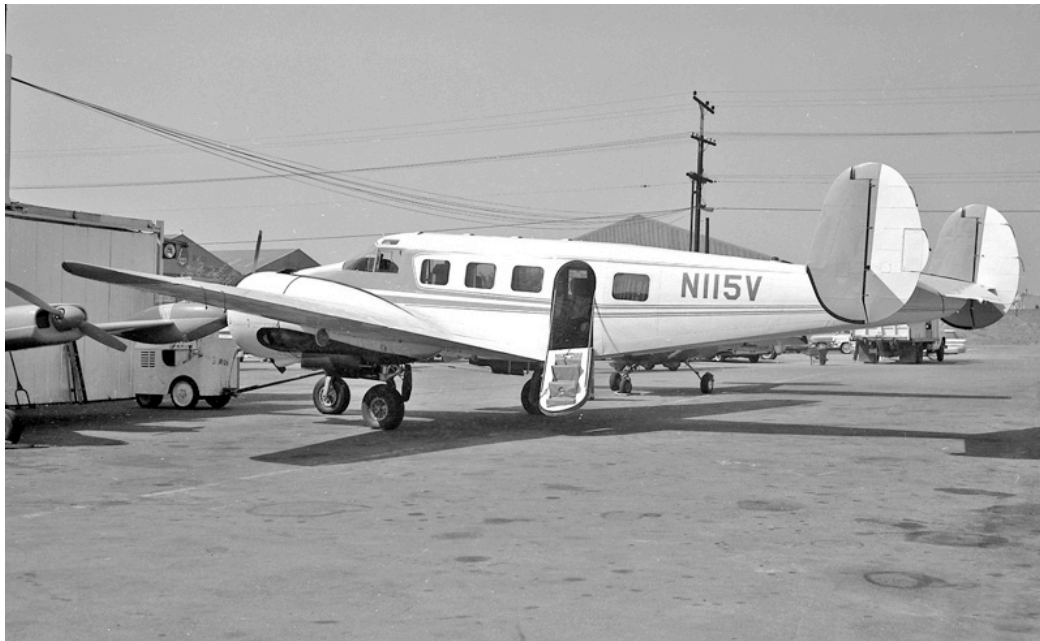
Civilianised C-45G N115V (AF-17) at Hawthorne Municipal, California in 1963. This aircraft has been fitted with Volpar trigear, wrap-around windscreen, enlarged windows and raised cabin roof. Photo by Eddie Coates
