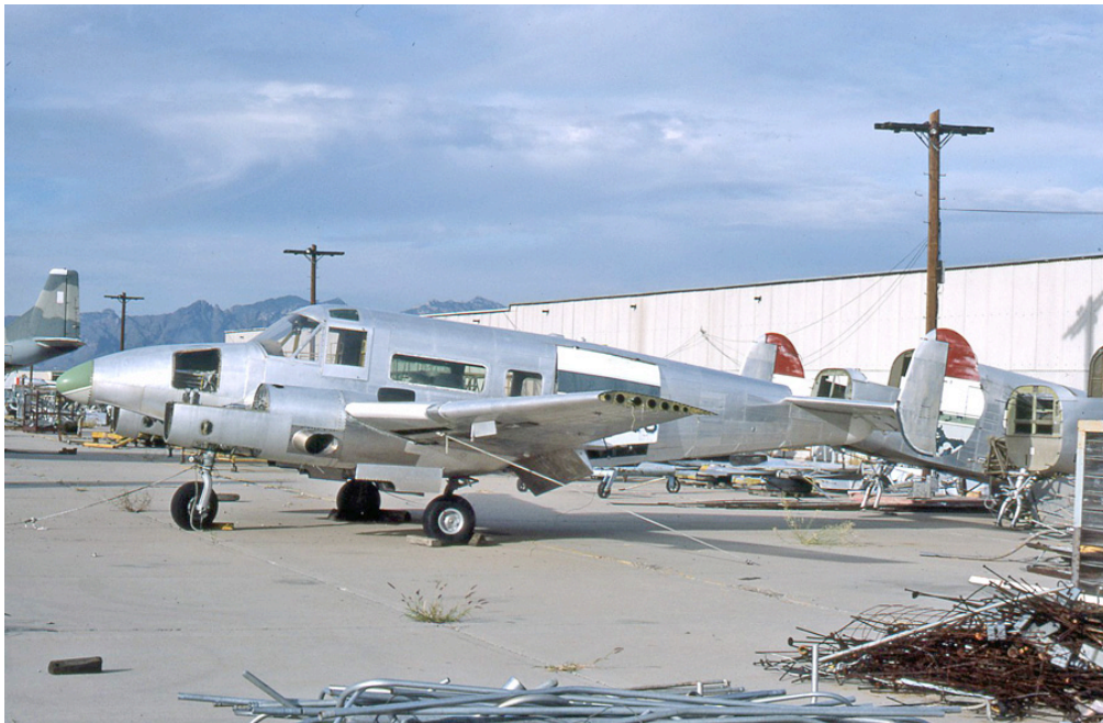
Uncompleted Hamilton Turboliners at Tucson AZ in October 1987 after the conversion line was shut down. Although fitted with E18S style high roof cockpits, these were probably from Hamilton Aircraft Co's stocks of retired military Beech 18 models listed above.
